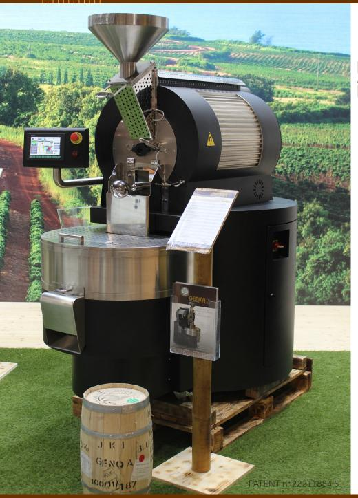
the first range of roasting machines with an induction system
