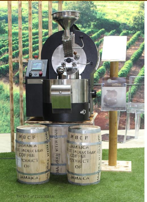
the first range of roasting machines with an induction system
